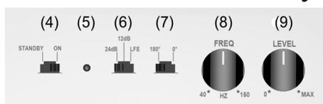
Adjust the filter's slope (6) according to your main speaker type: 12dB for sealed enclosure and 24dB for bass reflex enclosure.
