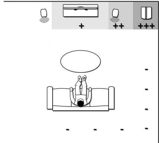
*A wall, and/or a corner, will naturally amplify the sound of your subwoofer, sparing work to the amplifier (compared to subwoofer in the center of the room with a fixed sound level: you gain +6dB against a wall, +12dB in a corner, knowing that doubling the amplifier's power only results in a gain of +3dB of sound level).*
